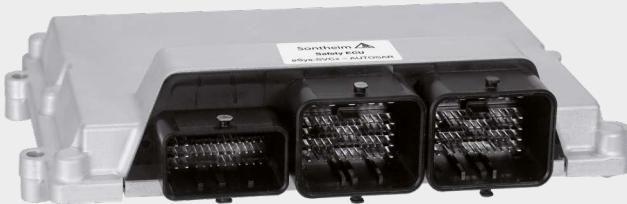
eSys-SVC3 is a powerful electronic control unit for safety-related applications up to ASIL-C. A rugged construction and a wide range of applications facilitate an optimal use in mobile machines. For this, three CAN, an optional LIN interface and up to 15 inputs and outputs with various diagnostic features are available.
